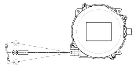
• To change the wire extraction direction, use special return pulleys
