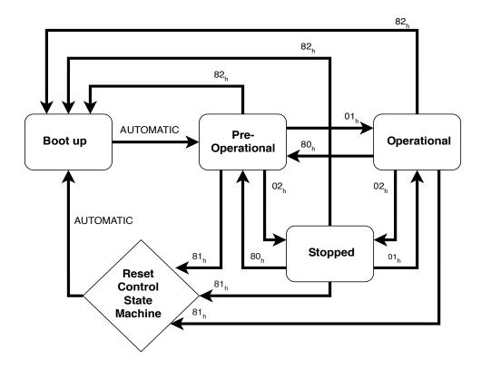
Every CANopen device contains an internal Network Management server that communicates with an external NMT master. One device in a network, generally the host, may act as the NMT master.
